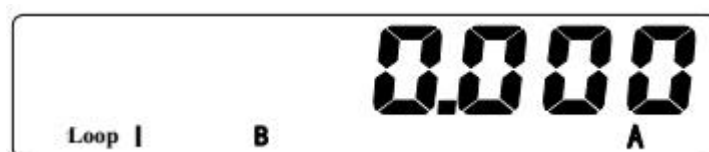
Figure 2 Phase B Current of 1st Circuit
