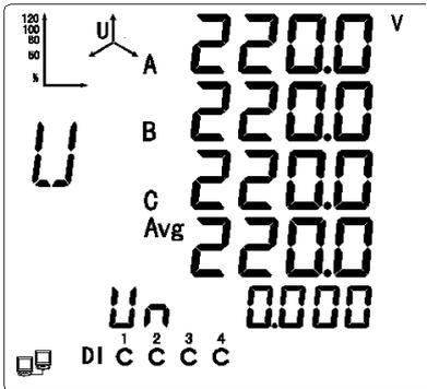
Press buttons “H” and “V/A” simultaneously at any display interface of metering data, it will enter the system setting interface.
