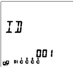
On communication address setting interface, the present communication address is 1.
