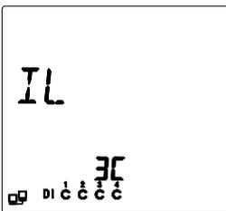
There are 3 options for the current wiring modes, i.e. “3C” referring to 3 CTs used for current wiring; “2C” referring to 2 CTs used for current wiring to calculate phase B current in three-phase balanced environment and “1C” referring to 1 CT used for current wiring to meter phase A current only, which equals to phase B current and phase C current separately in three-phase balanced environment.
