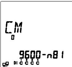
On communication parameter setting interface, the present baud rate is 9600. The RS485 communication parameter is n81.
