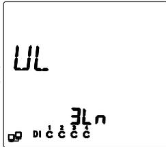
There are 3 options for the voltage wiring modes, i.e. “3Ln” referring to 3-phase 4-wire wiring mode; “2LL” referring to 3-phase 3-wire wiring mode, “2Ln” referring to 2-phase 3-wire wiring mode. The setting methods are as follows.
