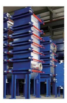
The crisscross of two plates is 180°. All plates are welded together and exchange heat through two short sides of each plate. As its gasket material utilizes the nonmetal materials which don't strech. So the medium temperature W400P, pressurew 3.0 Mpa. It expands the range of work, and also prolong the usage of cycle. What's more, reduce the expense of maintenance.
