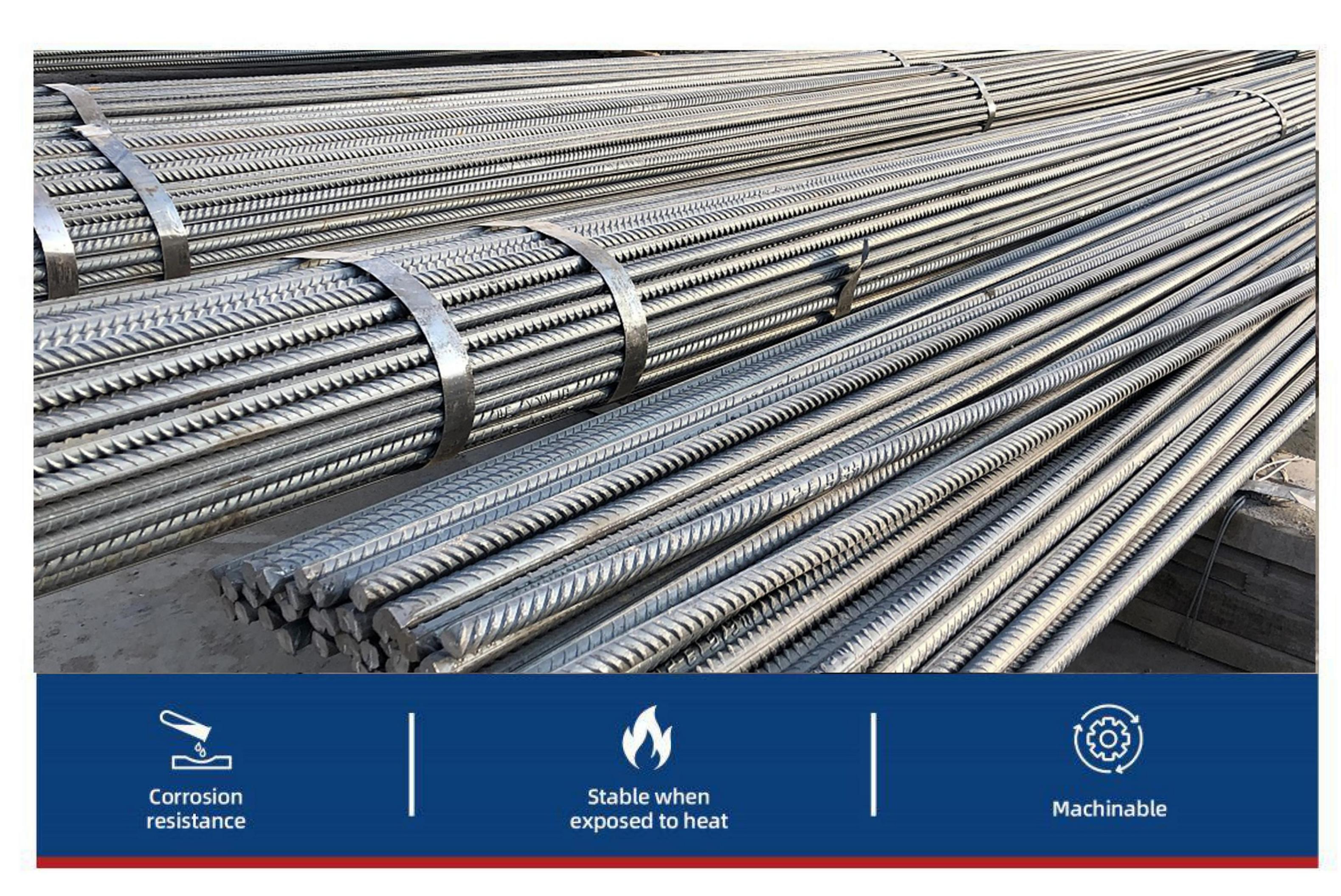
Steel bars mainly bear tensile stress in concrete. Due to the action of ribs, deformed steel bars have a greater bonding ability with concrete, and can better withstand external forces. Steel bars are widely used in various building structures. Especially for large, heavy, lightweight thin-walled and high-rise building structures.
