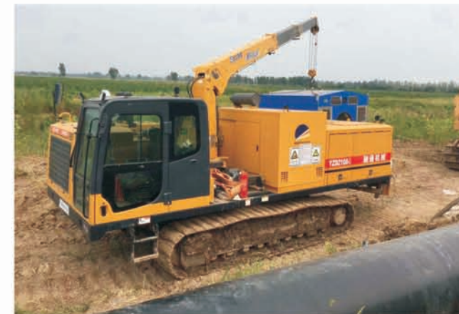
Project : 140kW mobile power station of multifunctional welding vehicle of CNPC Pipeline Bureau
